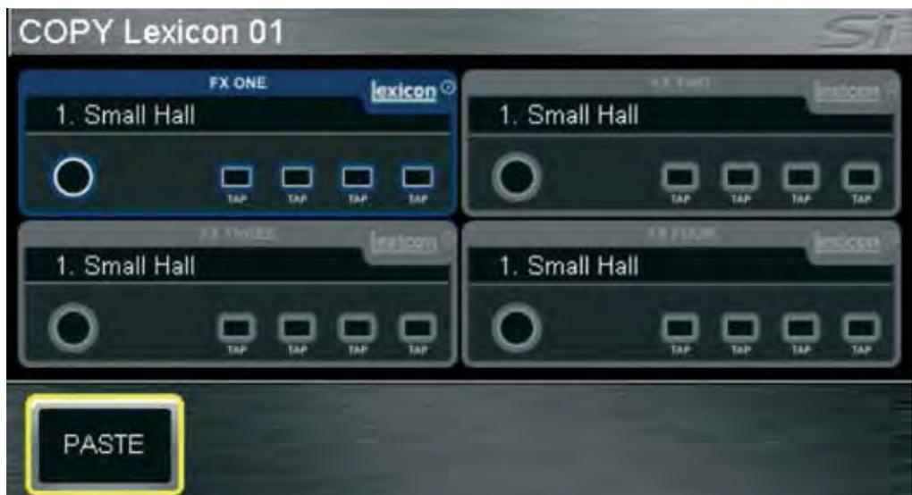
**Copy Lexicon settings between processors:** Pressing the FX key while in COPY & PASTE mode will display icons for all Lexicon processors; select the source processor by touching it's icon. To paste the processor press and hold the PASTE button while pressing FX'n' keys of the destination processors.
