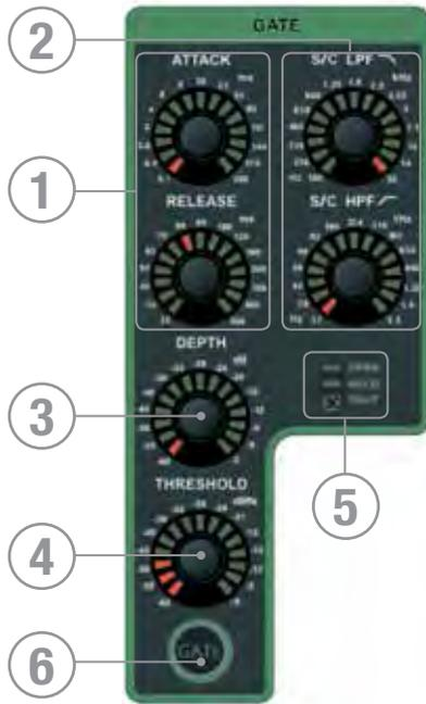
1. GATE ATTACK & RELEASE: indicates and adjusts the attack and release times of the gate.
