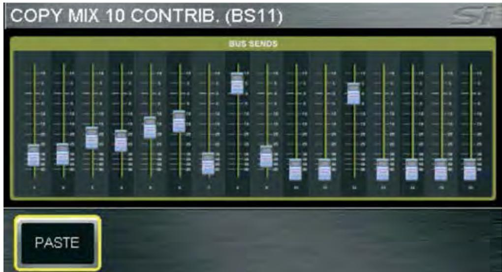
**Copy sends from all channels to bus'n':** Pressing COPY & PASTE while in FOLLOW mode or changing to FOLLOW mode while in COPY & PASTE will copy to the clipboard bus send levels and ON/OFF from all channels to bus 'n'. To paste the contributions from to another bus press and hold the PASTE button while pressing MIX'n' key(s) of the destination mixes.
