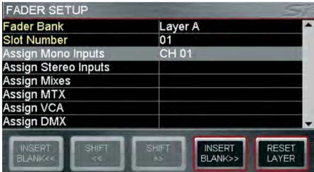
The fader setup provides a mean to define which channels (or buses) appear on which faders of which layers.
