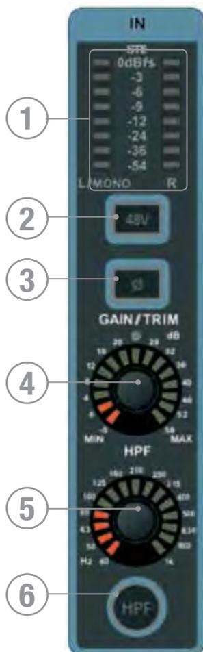
1. Meter: indicates the level in the channel or bus; if the source is MONO only the left meter will indicate signal, if the source is stereo the stereo indicator will light red and the meter will operate in stereo.
