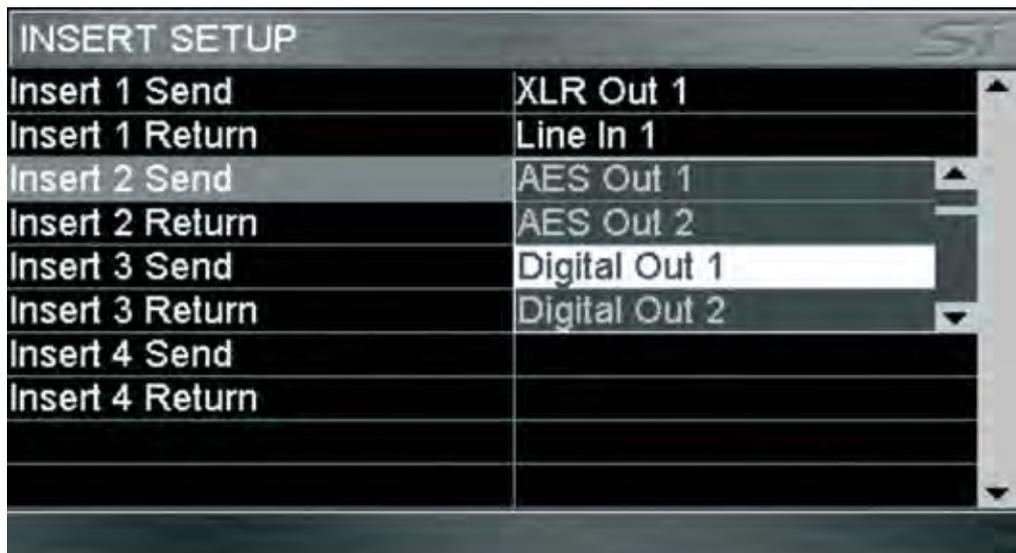
The inserts are configured from the INSERT SETUP button found on the INSERT screen. For insert sends, any line out or digital out channel may be used and for insert returns any line in or digital input may be used; once .
