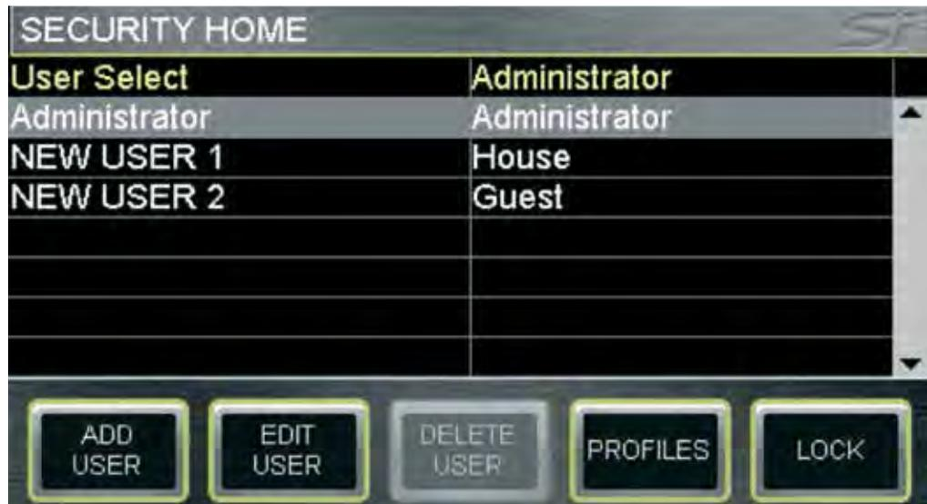
This facility allows some or all functions of the console to be locked preventing accidental or malicious misuse. All console settings may be easily locked at any time by pressing the LOCK button in the SECURITY menu.
