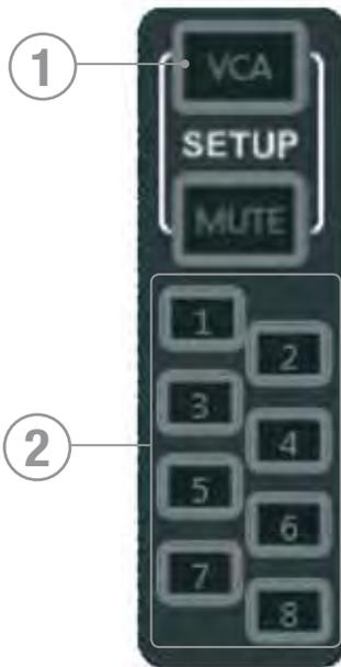
The VCA setup is enabled by pressing the VCA key, it then uses the mute masters in conjunction with input channel SElect keys to configure input channels as slaves to a VCA master.
