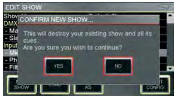
**LOAD:** Invokes loading of a new show from the internal Multi-Media Card (MMC-SD Card) or USB key if installed. Use the scroll/adjust encoder to navigate to the storage device and through the folder structures to select the file to load. The system will provide a warning that the action will overwrite the current show and allows the action to be aborted.
