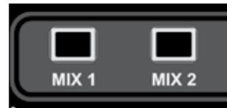
You may now open the GEQ for Mix 1 by pressing either the GEQ HI or LO key, close the GEQ by pressing the lit HI/LO key again.
