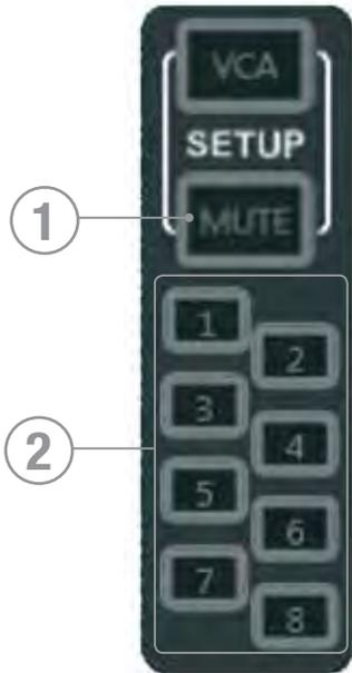
1. MUTE key: press this key to toggle in/out of mute setup mode; the key has no function on its own and requires the selection of one of the mute masters 1-8 to indicate which of the mute masters you are going to configure.
