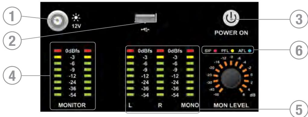
1. 12V LAMP OUT: Connector for LED or similar console light For use with 12v LED lights of under 100mA only! The intensity of the console lamps may be adjusted from the PREFS menu and some LED lamps supplied by Soundcraft incorporate a dimming switch on the lamp itself.
