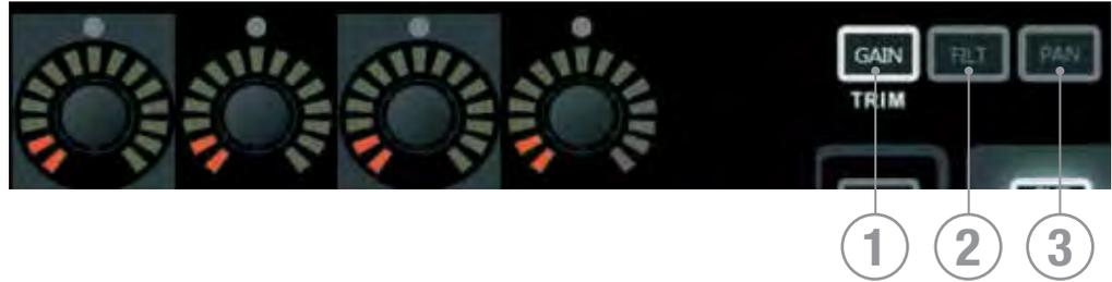
The Global Mode encoders offer control of a key parameter across all channels or buses currently active on the surface:
