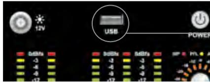
The Si PERFORMER software is updated via the USB port on the front panel. Details and special instructions for any release will be included with the software release package however the 'normal' procedure is listed below for reference:
