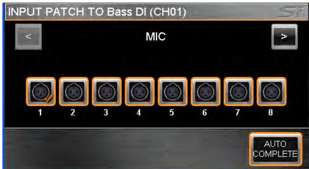
To have the system automatically patch multiple channels press the AUTO COMPLETE button; this will increment the input by 1 and patch by 1 until a logical group of patches is complete; see Auto Complete Boundaries for more information..
