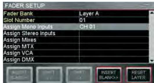
The following fields group the available processing channels, buses and controllers allowing easy selection of the channel bus or controller you wish to assign to the SElected slot, selecting any field will offer a drop-down list as follows:
