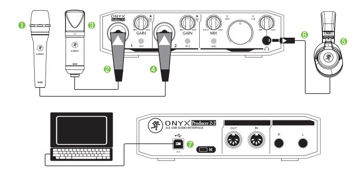
The **EM-91C** condenser microphone (1) is connected to channel 1 (2) and the **EM-89D** microphone (3) on channel 2 (4) of the **Onyx 2•2** interface. Check the **Onyx 2•2** manual for tips on getting gains and monitoring set up.
