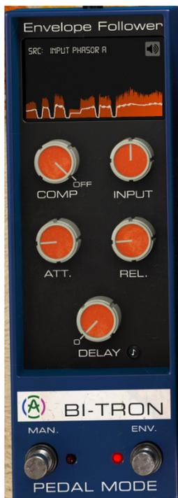
You have five controls for the Envelope Follower. The first one is a Compressor, which compresses the envelope generated by the source signal (the white curve on the graphic display) before using the contour as a modulator. The control actually acts as a threshold for a fixed compression ratio and its range goes from -60 dB up to 0 dB, and defaults to Off.
