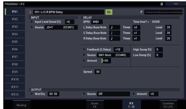
When you move the joystick away from yourself and press the SW1 button, the feedback level will increase, and the delay sound will continue for a longer time. The **Amount** setting specifies the feedback level that will be in effect when the SW1 button is pressed. If **Amount** is set to –10, pressing the SW1 button will reduce the feedback level to 0.
