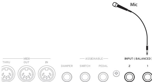
2. Adjust the Analog Input Setup dialog (SHIFT and AUDIO IN buttons) so that it's in the MIC position, and set the Analog Input Gain near the center.
