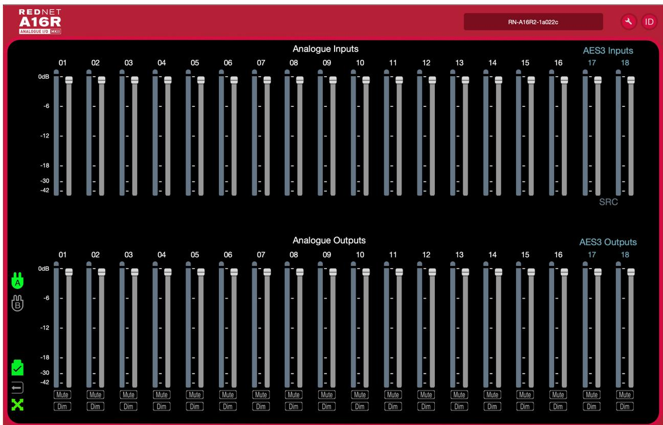
The image shows the Level control sliders, level meters and the Mute/Dim buttons for each of the 18 inputs and outputs.
