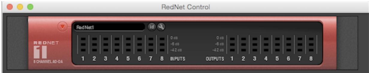
Expanding the RedNet PCIe/ PCIeR card inputs (vertical axis – **Dante Receivers**) and the RedNet 1 audio inputs (horizontal axis – **Dante Transmitters**) will give a display like this:
