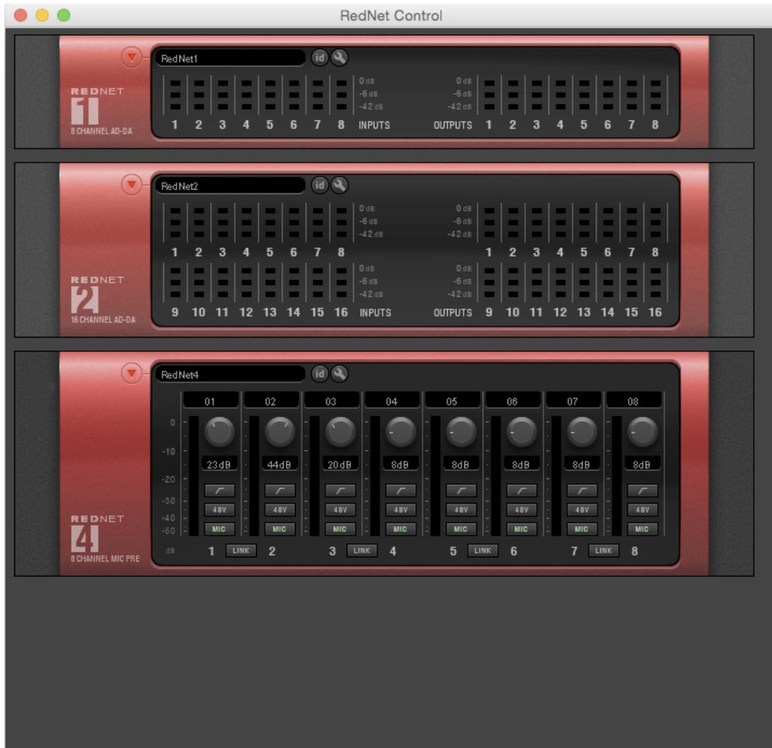
Each RedNet unit on the network will have a corresponding virtual front panel on-screen, so the display on your system will probably differ from that above, where the example system has one each of RedNets 1, 2 and 4.
