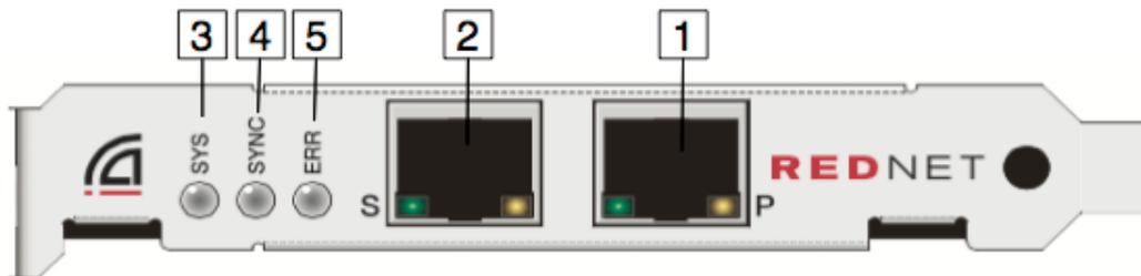
1. **Primary Network Port** - Connect this to the Gigabit network switch local to the computer. The port is the primary interface for all the channels of audio on the RedNet network. The socket has integral LEDs which illuminate to indicate connection to an active network port, and network activity.
