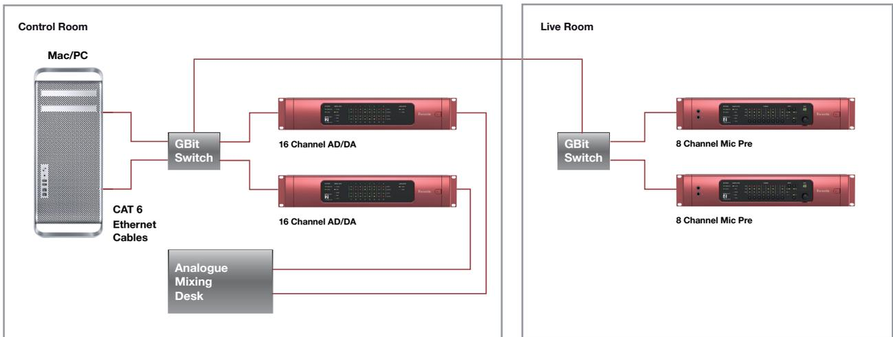
This small studio system would allow up to 48 sources to be recorded simultaneously; 16 of these could be from mic or line sources in the live room, with another 32 from line sources in the control room via the RedNet 2 units. Up to 32 outputs could also be made available via the RedNet 2's outputs.
