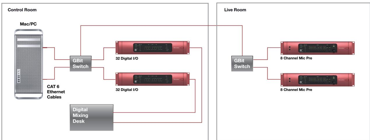
This would be a suitable system when the mixing desk in use was digital rather than analogue. RedNet 3 replaces RedNet 2 in System 2. This would provide up to 64 digital inputs into the system via RedNet 3's ADAT-format inputs. If analogue sources were required in the control room as well, a RedNet 1, 2 or 4 as appropriate could simply be added to the network.
