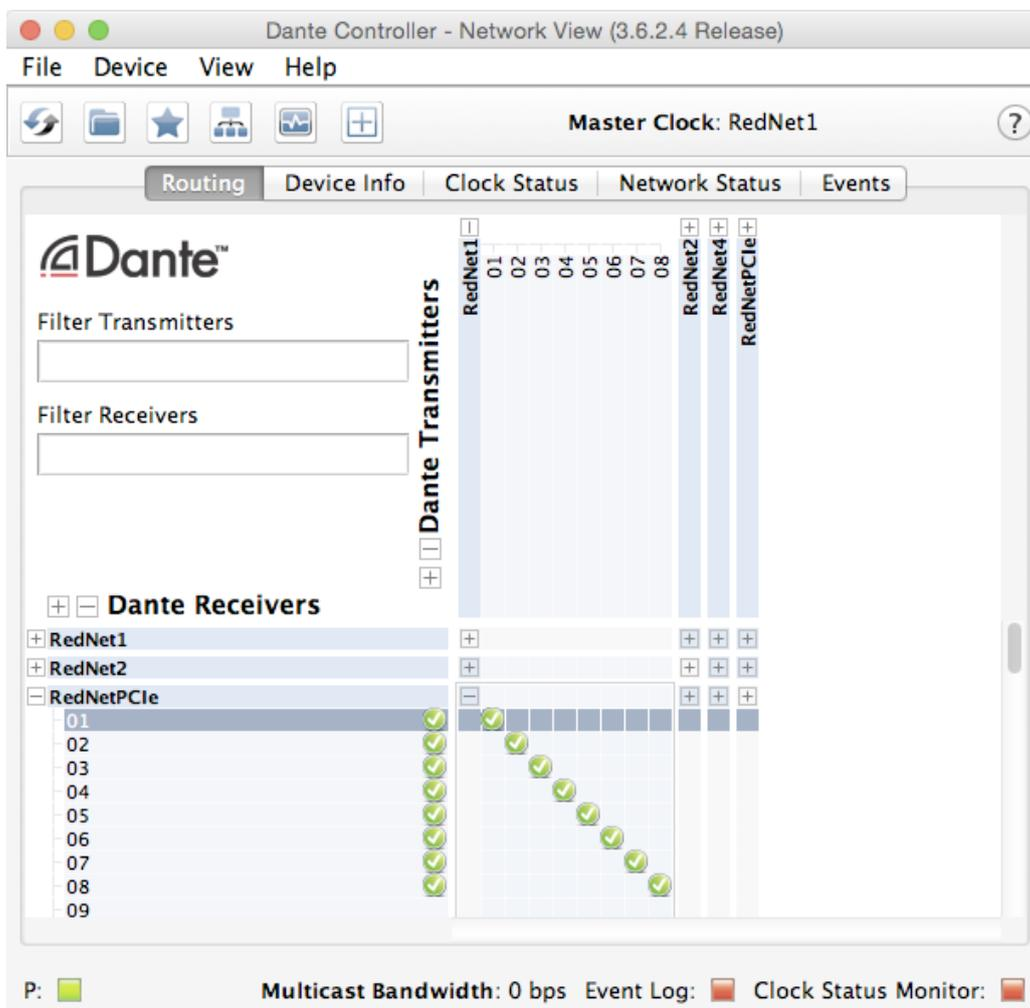
You can see that the Dante Controller confirms that each of the RedNet 1's analogue inputs 1 to 8 is mapped to the RedNet PCIe/ PCIeR card's network receive channels 1 to 8, by a green tick. Similarly, expanding the RedNet PCIe/ PCIeR card outputs (horizontal axis – **Dante Transmitters**) and the RedNet 1 audio outputs (vertical axis – **Dante Receivers**) gives a display like this:
