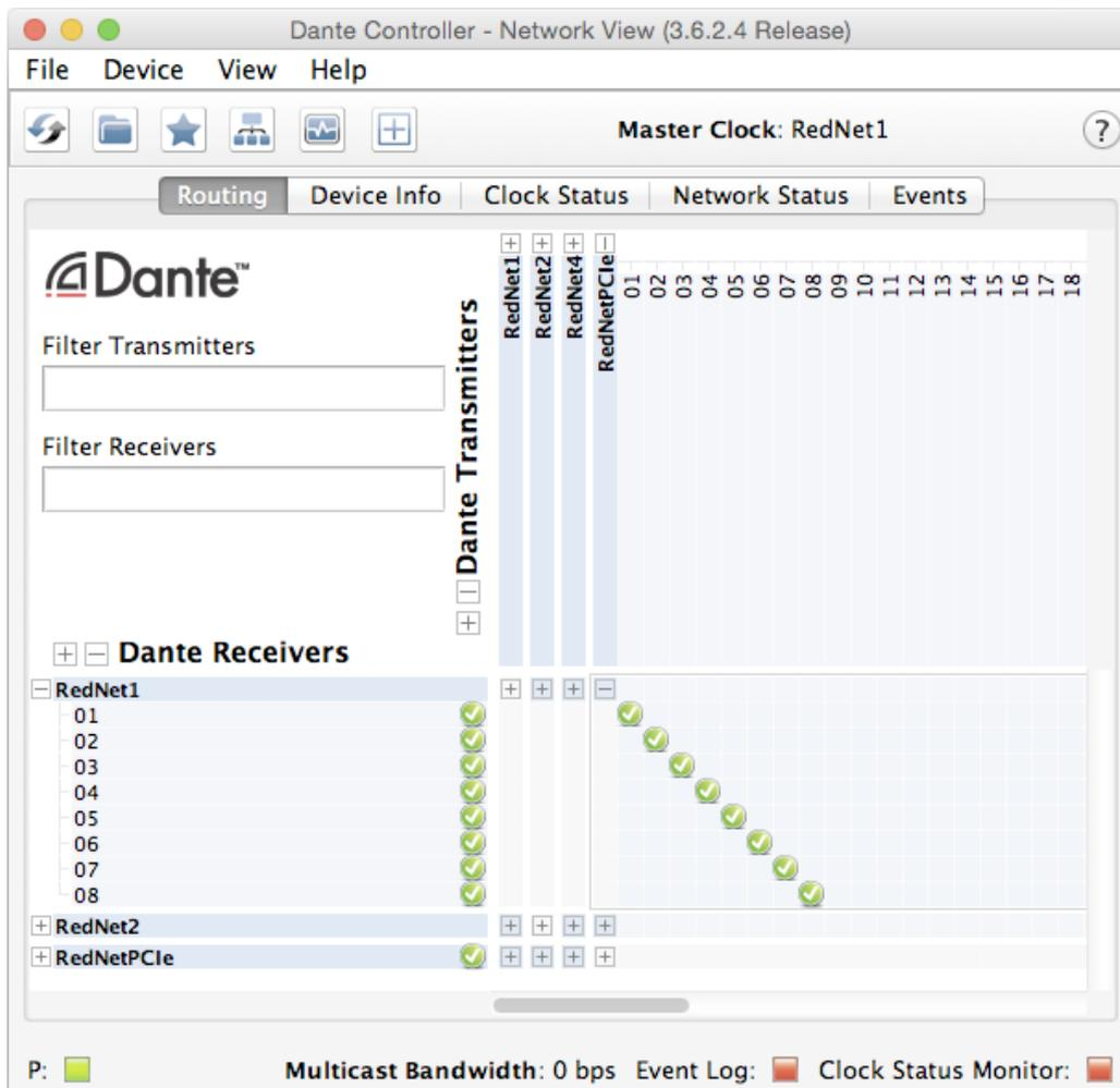
Again, Dante Controller confirms that each of the network transmit channels 1 to 8 of the RedNet PCIe/ PCIeR card is mapped to RedNet 1's analogue outputs 1 to 8.
