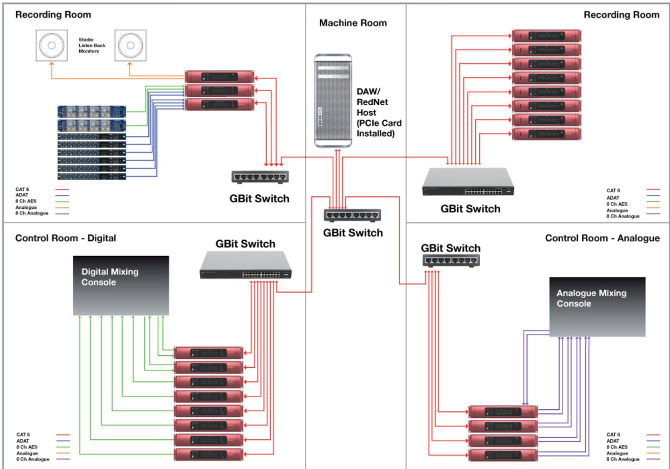
In this more complex, centralised system, users in any room would be able to access audio sources from any other room. Each room has its own local Ethernet switch, and each is connected in turn back to a central switch in the machine room. The host computer – which may or may not be a DAW platform – is connected to this central switch.
