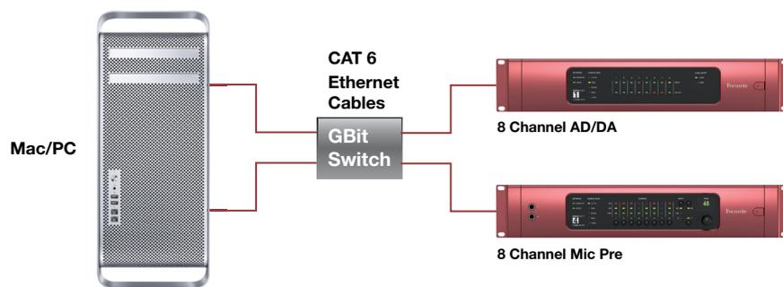
Using a simple system of two RedNet units, up to 16 sources could be simultaneously recorded, and up to 8 of them could be via the Focusrite microphone preamplifiers in the RedNet 4. Up to 8 outputs could be created for monitoring or downmix purposes.
