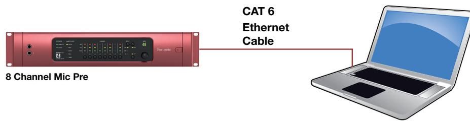
This shows the very simple network required if your system does not include a RedNet PCIe/ PCIeR card. The host computer would instead have the Dante Virtual Soundcard installed, and a single Cat 6 connection between RedNet 4 and the host's resident Ethernet port would suffice. This system would be ideal for basic high-quality recording but would require monitoring to be through an amplifier/ speaker system connected directly to the host computer's resident audio output.
