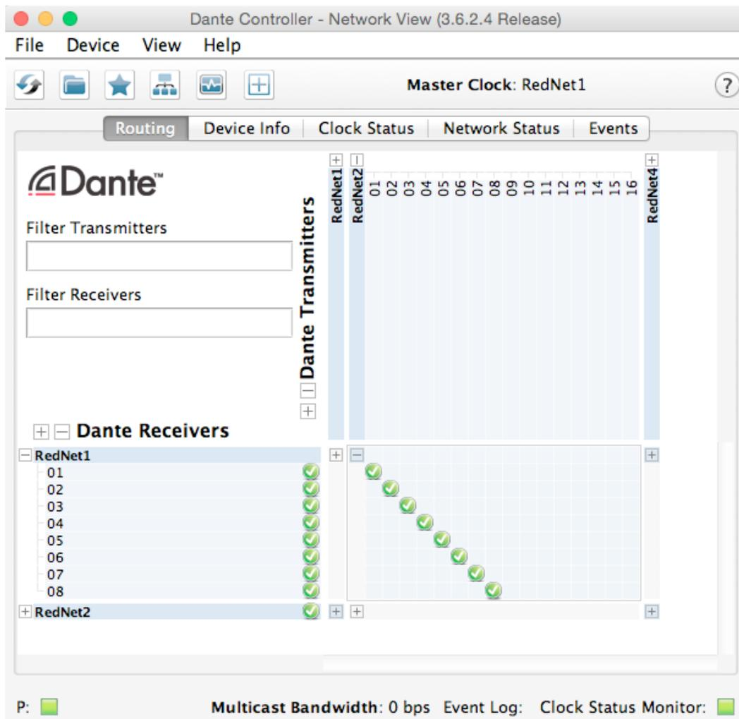
The Dante Controller window has five tabs; **Routing**, **Device Info**, **Clock Status**, **Network Status** and **Events**. The **Routing** tab is where custom audio routings can be set up.
