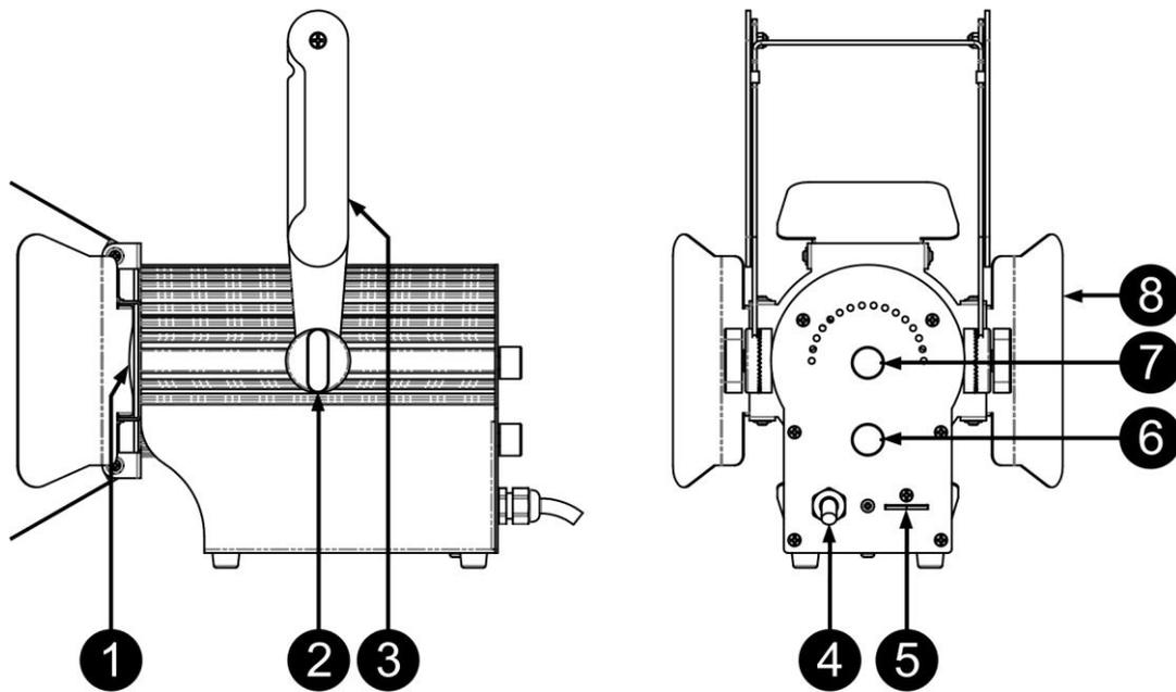
1. **MAGNETIC FILTERHOLDER:** to hold different kinds of filters with a diameter of 7cm.
