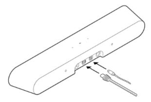
Connect the optical cable to your TV's optical digital OUT port.
