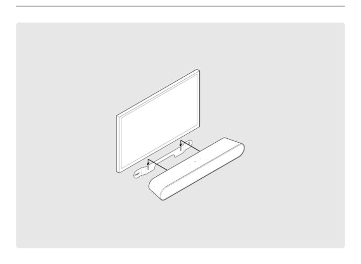
If your TV is wall-mounted, align the top edge of the bracket with the bottom of your TV, leaving at least 2.5 inches (mm) between them.
