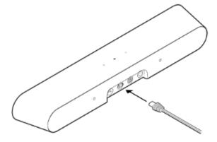
Connect the optical cable (included) to the optical port on the back of your soundbar.
