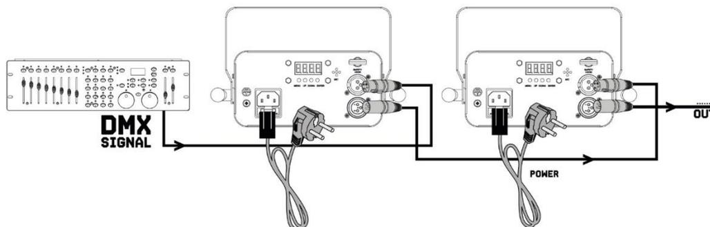
**CAUTION!** At the last unit, you must close the DMX line with a terminating resistor. Take an XLR connector and solder a 120 Ohm resistor between signal (-) and signal (+) and connect it to the DMX output of the last unit in the line.
