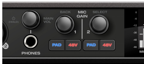
Figure 5-2: Push the knob to activate the functions labeled in gray.
