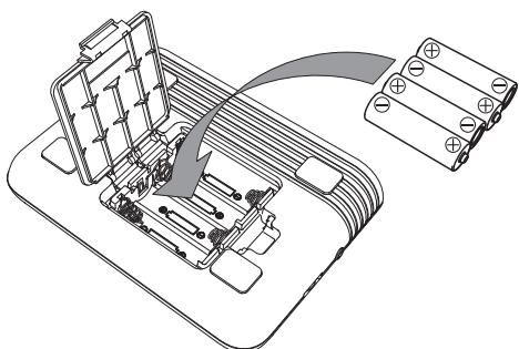
**Note:** When the batteries run low, **BAT** blinks on the display. Please replace the batteries.
