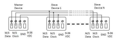
Interfaces configured as slave will strictly follow the clock, triggers and information providing by the master interface. Only one master interface at a time.
