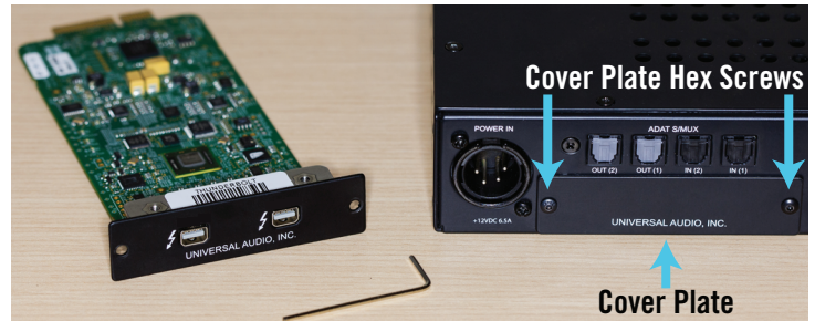
Items gathered and ready for installation (the appearance of your option card may differ slightly)
