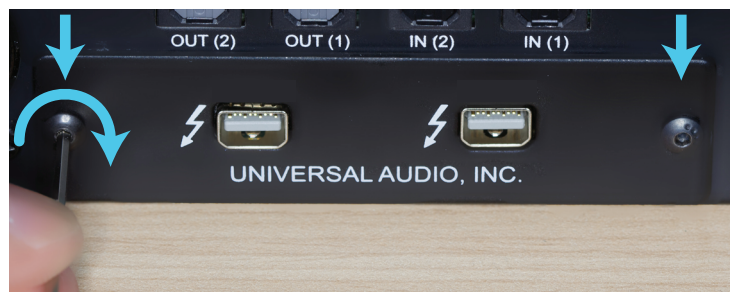
Secure the option card with the two saved hex screws
