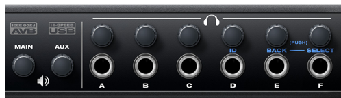
Figure 6-2: Push the knob to activate the functions labeled in blue.
