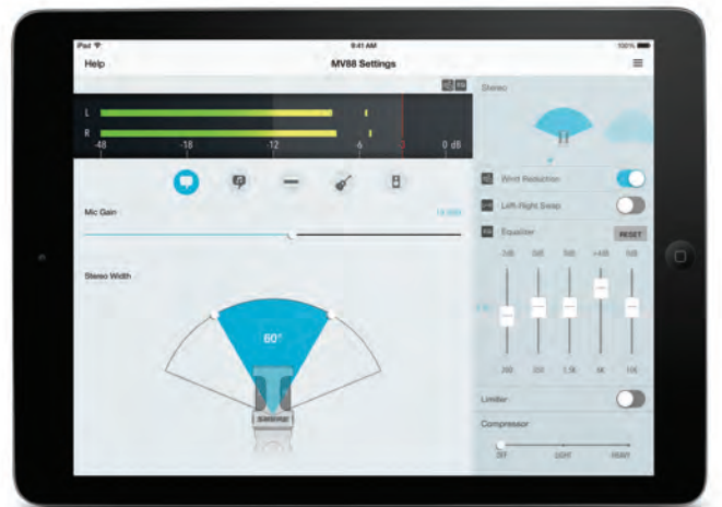
MV88 Advanced Settings Screen Polar Pattern Select, 5-Band EQ, Wind Reduction, Compressor, Limiter, Left/Right Channel Swap
