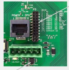
DMX CHIP Solder the DMX chip to the 8 pin connector on the right of the RJ45 socket. Be sure that the chip is facing downwards
