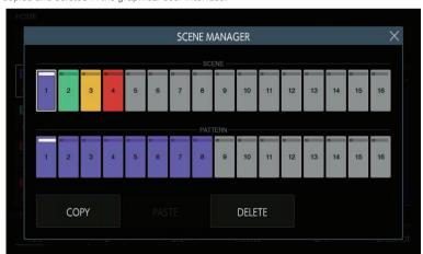
Each scene has its own unique color, and the patterns within a particular scene are also represented with the same color as the scene. The LEDs of the 16 step keys of the hardware also light in the same colors when the mode is switched to SCENE/PATTERN selection mode. Tapping the [X] button at the top right of the display or pressing the [BACK] button closes the screen.
