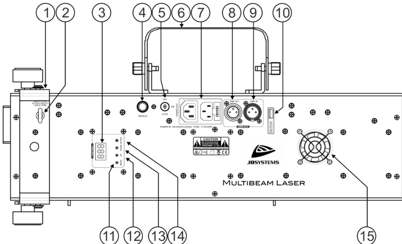
1. **HANGING BRACKET** : for hanging the Multibeam Laser in vertical position.
