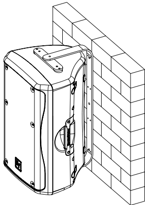
Kits Used - MB5 Wall/Ceiling Mounting Bracket (Wall Configuration)
